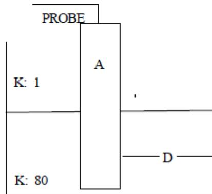
If the tank is filled with water ( $K = 80$ ), it displaces air ( $K = 1$ ), and we have a dramatic change in capacitance which is utilized in the electronics to activate a relay or transmit a signal proportional to the amount of water in the tank. The electronics allow for tuning of the system so that the operator can activate a relay at any point or measure between a wide choice of spans.
